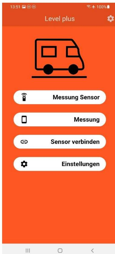
After starting the app, you will be taken to the main page (Home). You can only start a measurement with a sensor here if you have previously established a connection to a sensor. To do this, select "Connect sensor".
