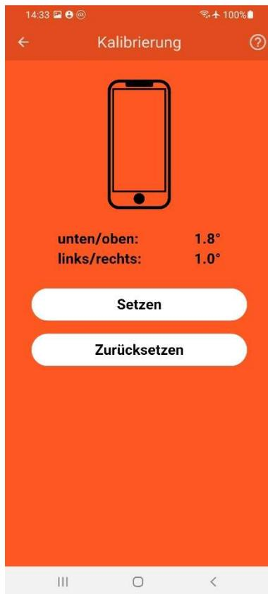
The smartphone or tablet can be calibrated in Level pro and Level plus. If the smartphone or tablet does not have a level surface or does not display a horizontal plane accurately, you can calibrate the device. To do this, place the device on a level surface and press "Set".
