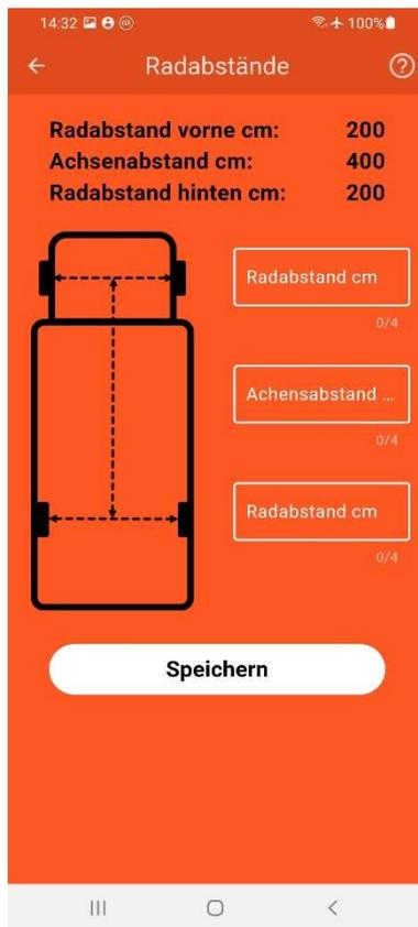
Only in the Level plus and Level pro apps can the wheelbase of your vehicle be entered and saved so that a height correction can be calculated individually.
