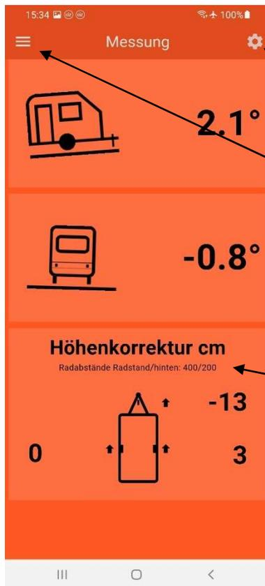
In the upper section, the inclination of the vehicle from rear to front and the inclination from left to right is displayed in degrees in the interval  $[-30^{\circ} \text{ -- } +30^{\circ}]$ .
