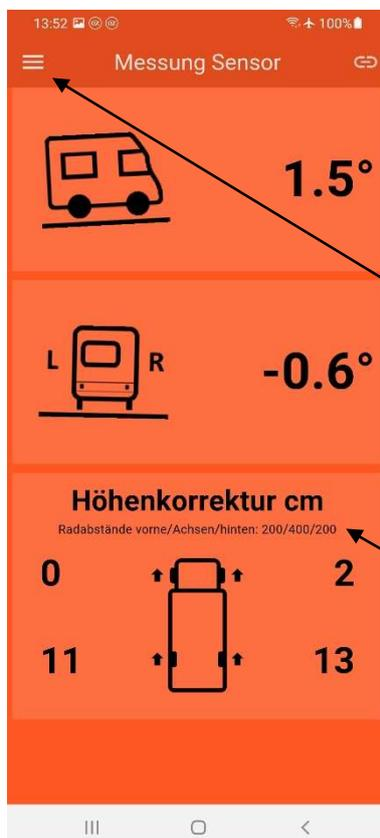
In the upper section, the inclination of the vehicle from rear to front and the inclination from left to right is displayed in degrees and in the interval [-30° - +30°].
